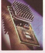
The Doubler 4000 includes an on-chip math co-processor, and will dramatically speed up any application - such as rendering - that depends on calculations. It is completely reliable and system safe. An integral cooling system ensures that the Doubler 4000 runs cooler and more reliably at 50 MHz than the original processor.
