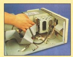
Take one of the ribbon connectors and line up the pins on the back of the drive with the ribbon connector's holes.
