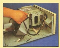
Take any one of the power leads. These are easily distinguishable – they're the ones with multi-coloured wires going in. Do the same as with the ribbon connector and push it firmly on to the drive.
