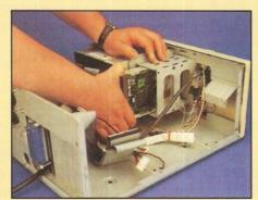
Slot the drive into one of the bays. If you prefer you can unscrew the bay easily and remove it to fit the drive externally.
